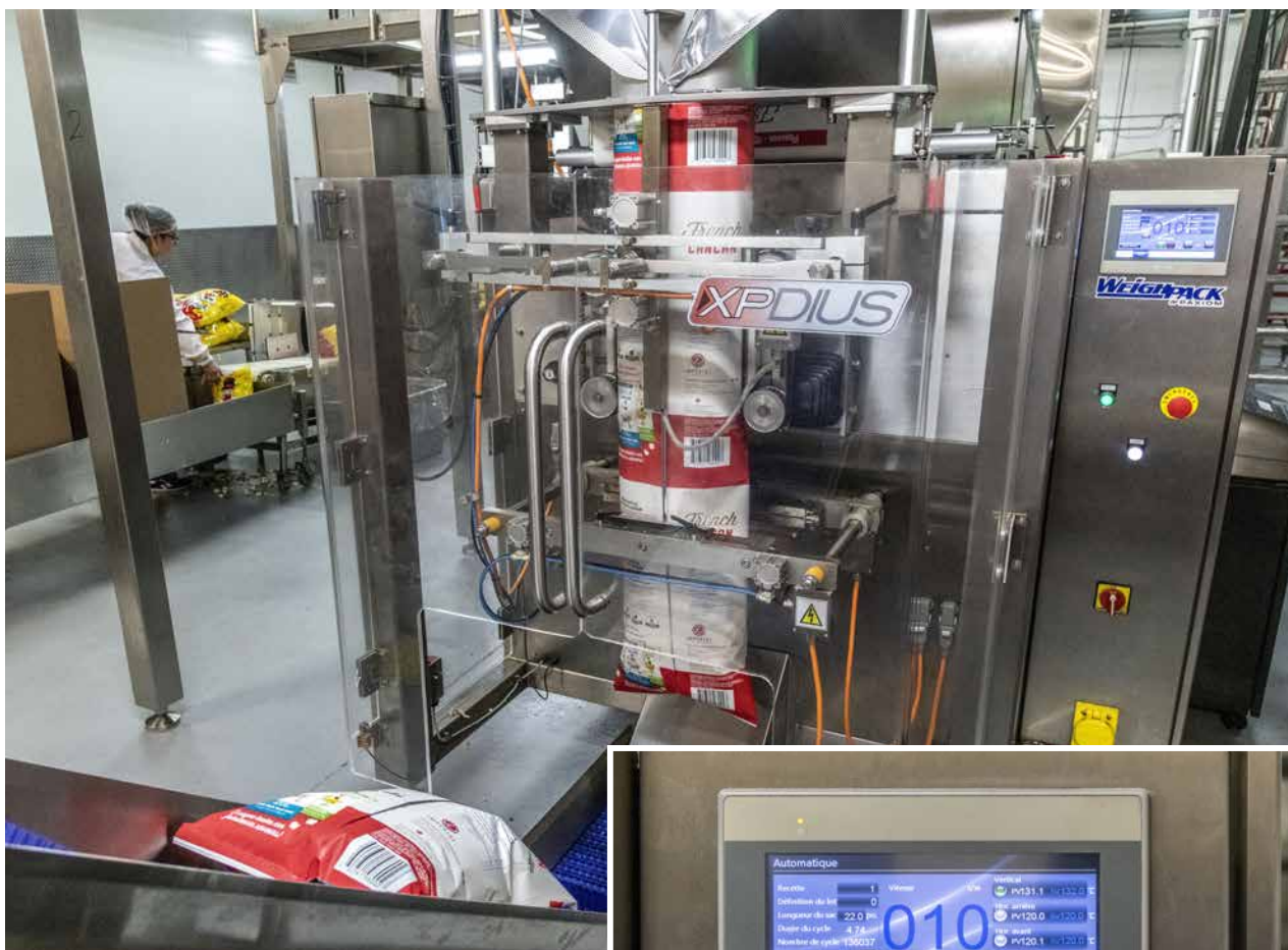
Featuring a built-in touchscreen HMI (human-machine interface) near the top of the electronic controls cabinet to provide easy programming and monitoring for machine operators, the WeighPack brand XPDIUS Elite vertical form-fill-seal machine uses specialty metallic foil bags to package the French Cancan line of premium-quality popcorn products at speeds of 10 to 12 bags per minute in perfectly-controlled continuous workflow that ensures nine-month shelf-life for the bagged popcorn.
