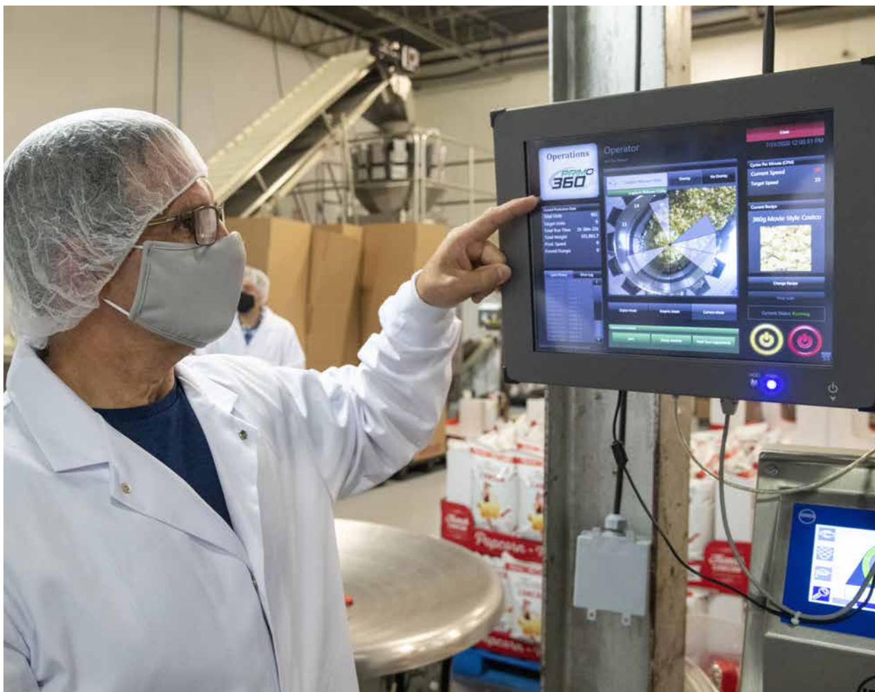
The fully-automatic 14-bucket PrimoCombi weighscale at the Imperial Snacking production facility is capably supported by the 360 operating system that enables operators to create reports, event logs, archives or production results, and to provide production analysis to ensure optimized production workflow and production efficiency levels for the busy plant.
