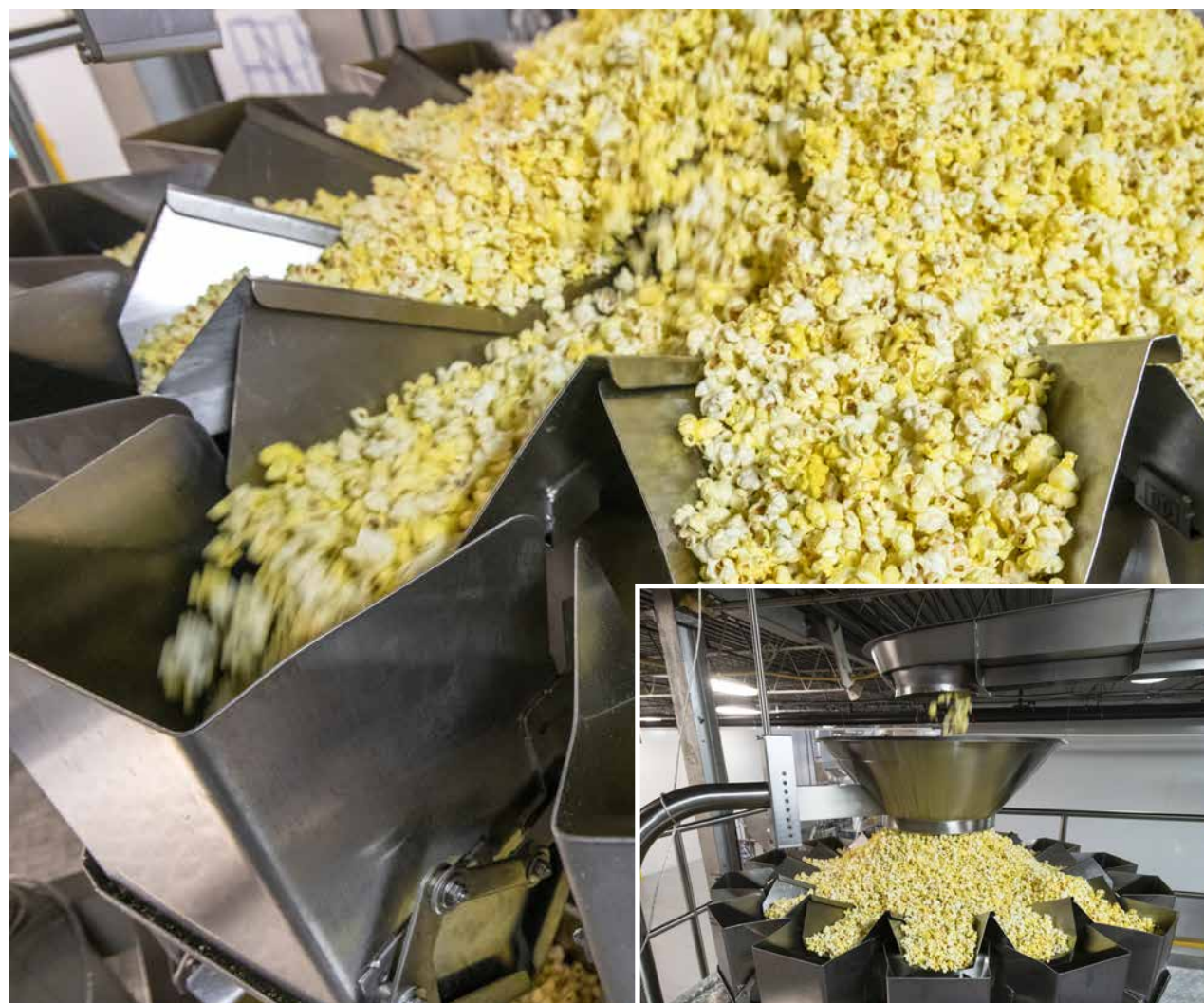
Installed at the mezzanine level, the 14-bucket PrimoCombi automatic weighscale supplied to the Imperial Snacking plant by Paxiom Group delivers superior accuracy and weighing precision in delivering smooth and consistent flow of the lightweight fluffy product to all of the system's vibratory feeder pans and the stainless steel buckets that automatically dispense the precise quantity of product down to the bagging machines on the ground floor below.
