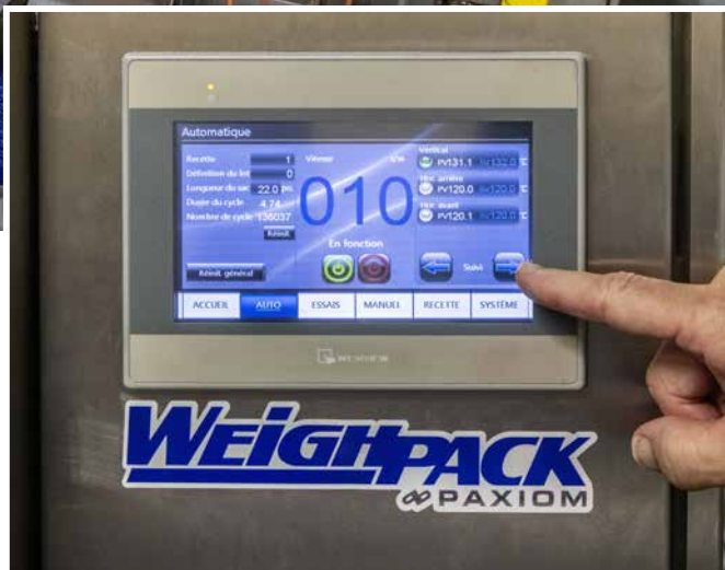
Featuring a built-in touchscreen HMI (human-machine interface) near the top of the electronic controls cabinet to provide easy programming and monitoring for machine operators, the WeighPack brand XPDIUS Elite vertical form-fill-seal machine uses specialty metallic foil bags to package the French Cancan line of premium-quality popcorn products at speeds of 10 to 12 bags per minute in perfectly-controlled continuous workflow that ensures nine-month shelf-life for the bagged popcorn.
