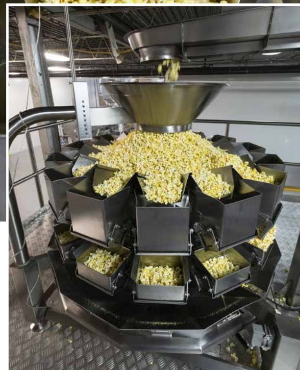
Installed at the mezzanine level, the 14-bucket PrimoCombi automatic weighscale supplied to the Imperial Snacking plant by Paxiom Group delivers superior accuracy and weighing precision in delivering smooth and consistent flow of the lightweight fluffy product to all of the system's vibratory feeder pans and the stainless steel buckets that automatically dispense the precise quantity of product down to the bagging machines on the ground floor below.
