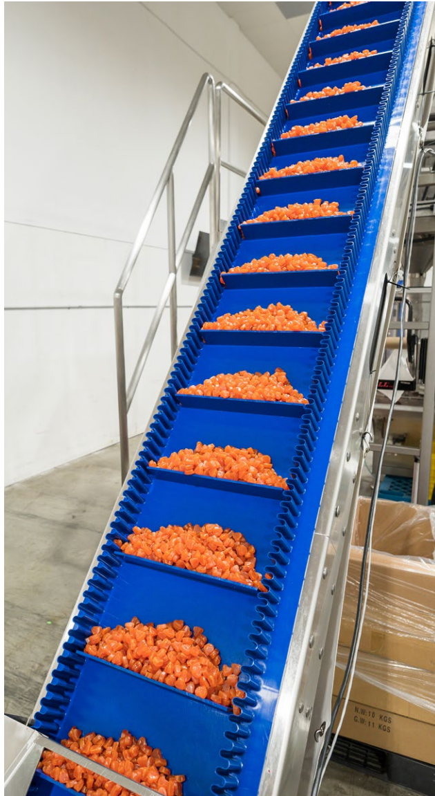
From left: An incline bucket elevator carrying pre-measured quantities of bulk gummies up to the mezzanine level to be dispensed inside the PrimoCombi multihead weigh-scale (center), which then dispenses the proper quantities of gummies down into the SpinDexer rotary container filling system (below)
